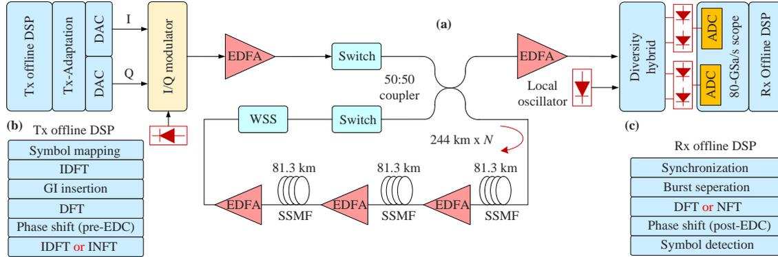
Figure 2: (a) General experimental setup NFDM transmissions over SSMF with EDFA-only amplification; (b - c): Transmitter (Tx) and receiver (Rx) DSPs; DFT (IDFT) – discrete (inverse) discrete Fourier transforms; NFT (INFT) – nonlinear (inverse) nonlinear Fourier transforms; EDC – electrical dispersion compensation; GI – guard interval.
