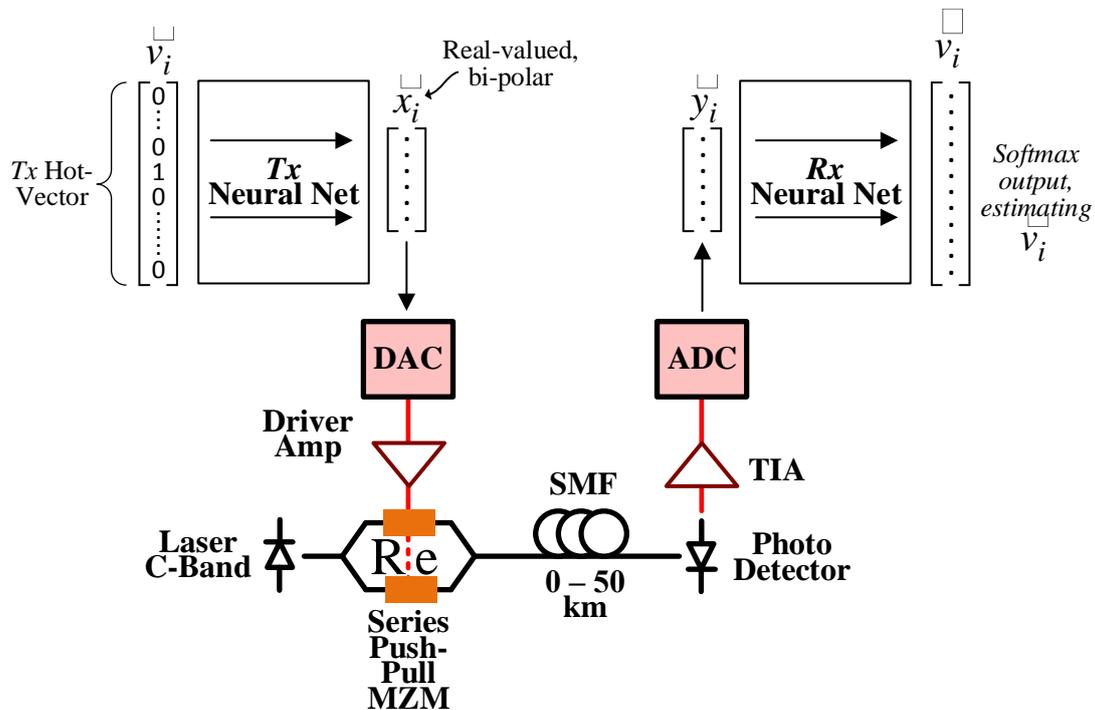
Figure 4: Schematic of the experimental test-bed, and how it interfaces with the dual transmit-receiver (Tx-Rx) Neural Networks.
