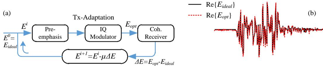
Figure 3: (a): Block diagram of the transmitter (Tx) adaptation routine; b) a comparison of the ideal and the generated signal
