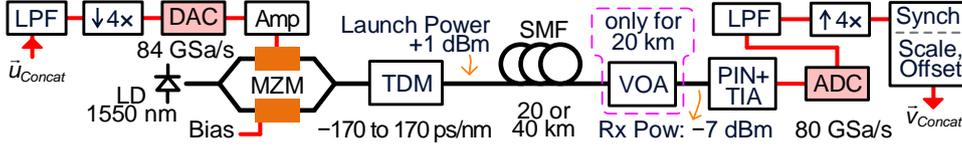
Fig. 2. Experimental testbed
