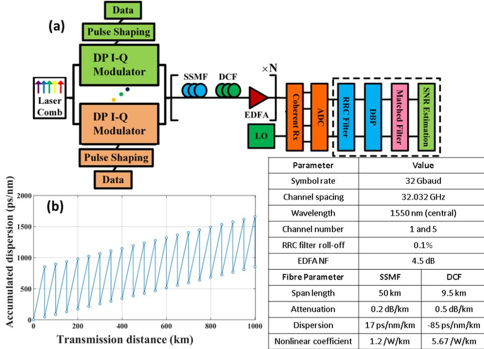
Fig. 1. Multi-channel DM transmission system simulation using DBP (a) LO: local oscillator, ADC: analogue-to-digital converter, N: number of spans. (b) Dispersion map. Inset table: system parameters.
