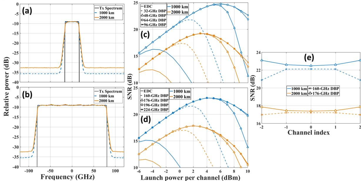
Fig. 2. Spectral broadening effect (4 dBm/ch) for (a) single-channel (32 GHz) and (c) 5-channel (160 GHz) transmission and (b) its impact on the SNR as a function of launch power for single-channel and (d) the outermost of 5-channel systems using DBP. (e) SNR versus channel index in 5-channel system for different DBP bandwidths. Power (optimum for central channel) is 3 dBm (160-GHz DBP) and 4 dBm (176-GHz DBP).
